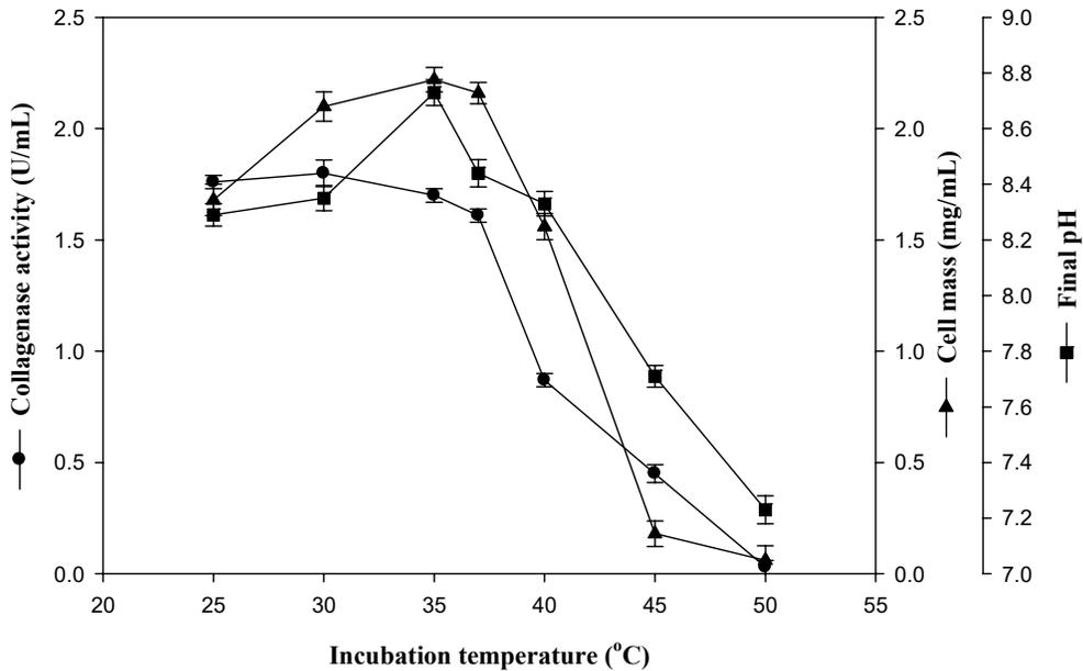
**Fig. 5.** Effect of incubation temperature on production of collagenase from *C. contaminans*
