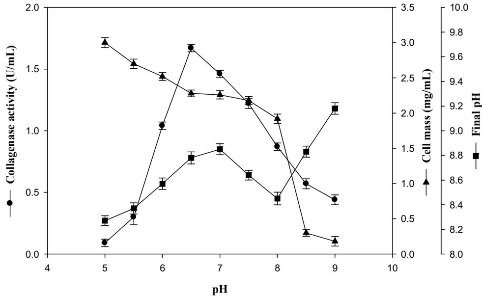
**Fig. 4.** Effect of medium pH on production of collagenase from *C. contaminans*
