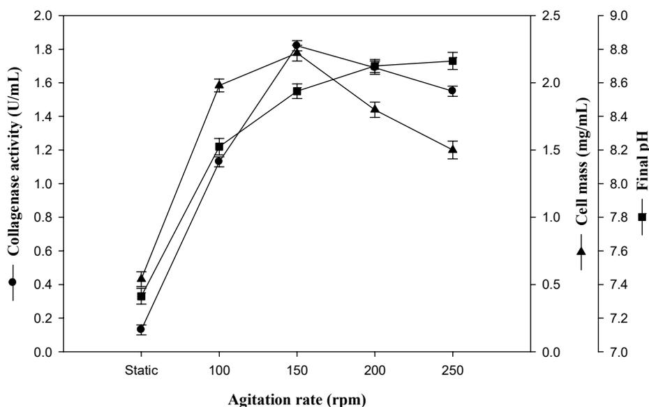
Fig. 6. Effect of agitation rate on production of collagenase from *C. contaminans*
